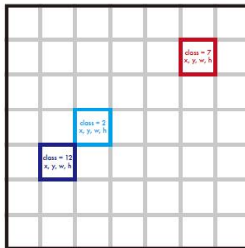
Train The Network To predict this grid of class probabilities and bounding box coordinates.
